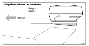
The shims may be made from aluminium plate wedges, simple flat washers, or an angled wooden block. For thick shims, you may need longer securing bolts than the M8x40 bolts supplied with the radome scanner, or the M10 studding supplied with the open array scanners.
